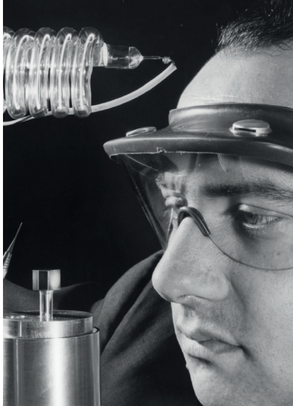
Theodore H. Maiman of Hughes Aircraft Company showing a cube of synthetic ruby crystal, the material at the heart of the first laser
