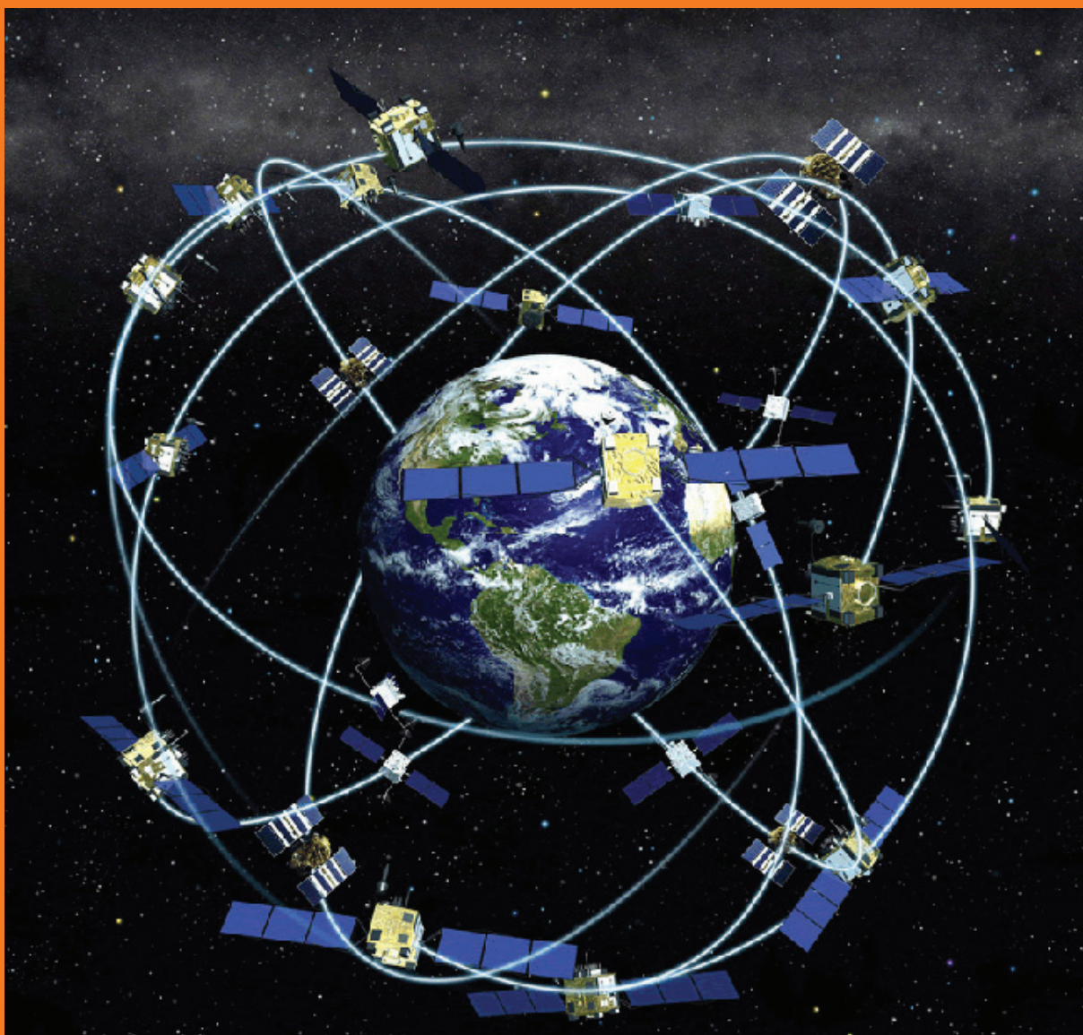
The GPS signal comes from a constellation of satellites in permanent orbit around the Earth. The timing needed to emit a precise GPS signal is provided by ultrastable atomic clocks mounted on board of each of the satellites
